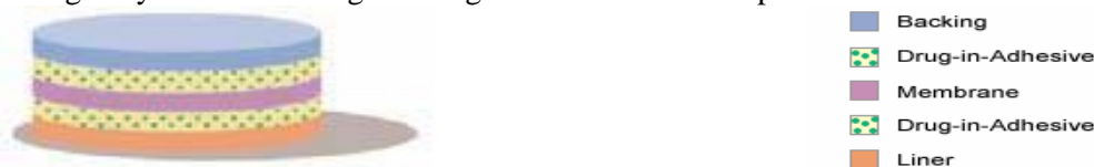
Figure.3. Multi-layer drug in adhesive patch and its different components
