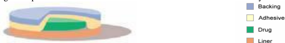
Figure.5. Single layer drug in adhesive patch with its different components
